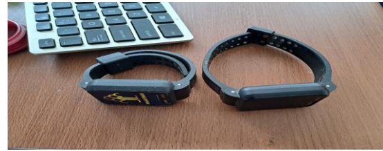
Figure 1. Inmate activity monitoring bracelet
